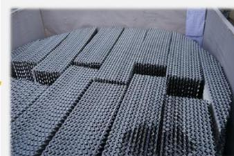
Coalescer – separation of water-methanol mixture from condensate stream
