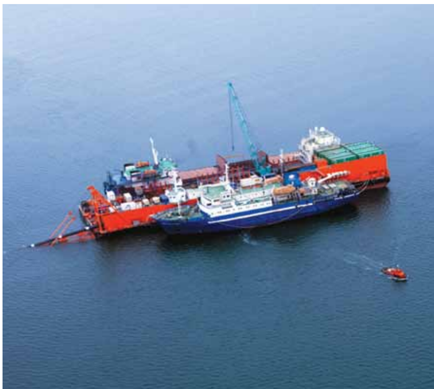
Defender pipe-laying vessel operating in Baidarata Bay
