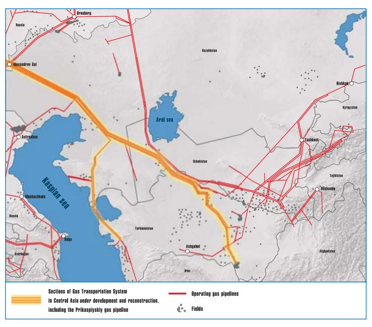
Gas transportation facilities will be constructed between the Belek compressor station (Turkmenistan) and the Alexandrov Gai gas measuring station (Russia) involving the reconstruction of the existing Okarem-Beineu gas pipeline (Central Asia-Center III) to transport Turkmen and Kazakh natural gas through the territories of Turkmenistan, Kazakhstan, and Russia.
