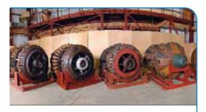
The complex of intrapipeline defectoscope produced by ZAO NPO "Spetsneftegaz" with the caliber of 1,400 mm.
