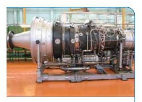
Drive Engine AL-31ST produced by OAO NPO "Saturn". Gazprom has established a technological base for the comprehensive reconstruction. It created and installed new types of gas pumping units at the compressor stations with efficiency up to 35 %. The following new engines are now in serial production: PS-90, AL-31ST, NK-36, D-336, etc. A total of 17 gas pumping units were replaced by new generation units and 1 gas pumping unit was upgraded in 2005.
